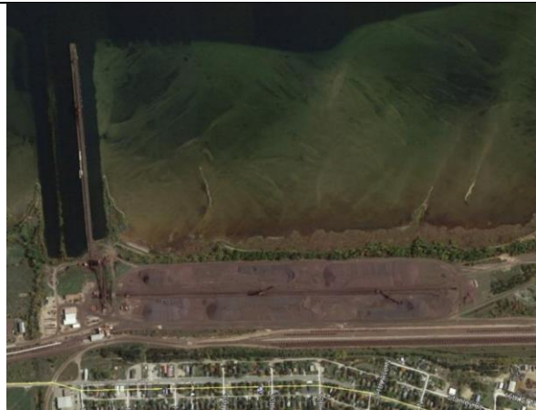
The last ore dock in Escanaba, Michigan was closed in 2017. It had replaced earlier conventional docks and utilized a conveyer system to load boats from a storage yard. (Google Earth 2013 image)
